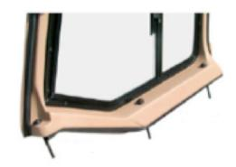
As you tighten the bolts, from the top of the insert, pull in, until they are snug. DO NOT OVER TIGHTEN.
