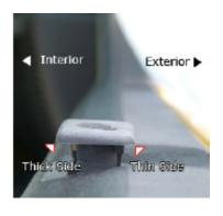
Install the new door inserts back into the lower door holes. There is a tab on one side of the insert, it can only fit into the hole in one direction. If the inserts are installed properly, the top plastic flange will rest against the top portion of the door.
