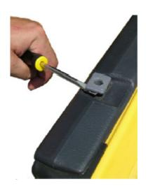
Once loose, the door inserts can then easily be removed by hand. There should be three (3) per side. Next run a screw driver bit down each hole about 6". Make sure the hole is not obstructed. Some YJ's have a plate at the bottom of the hole. You might need to run a 7/16" drill bit to clear the hole.
