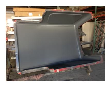
Spray in gelcoat which gives color to the fiberglass and helps release the part.
