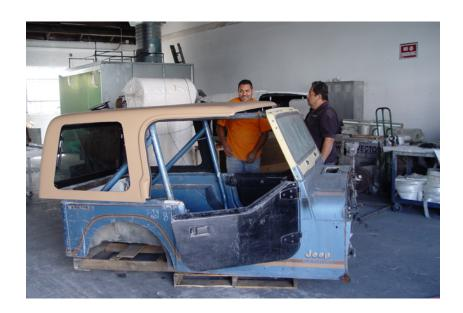
Test fit on Jeep and install all connection fittings.
