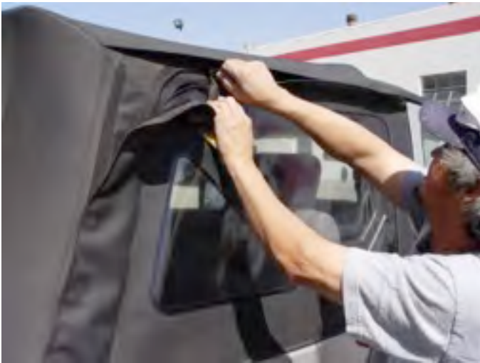
1. Remove side windows. (Left & right)
