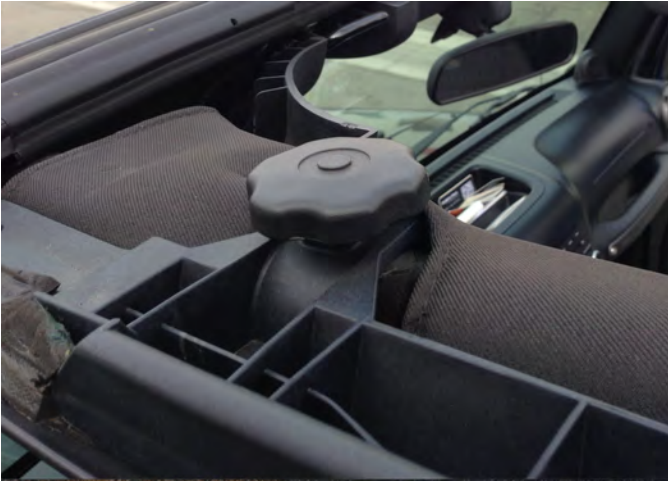
7. Unscrew the 3 attach knobs along each side. (Left & right)
