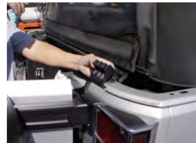
5. Remove retainers. (Left & right)
