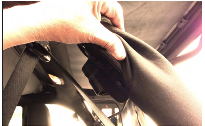
10. Disengage soft top mechanism at diagonal roll bar mount and remove mount. Remove soft top from vehicle.
